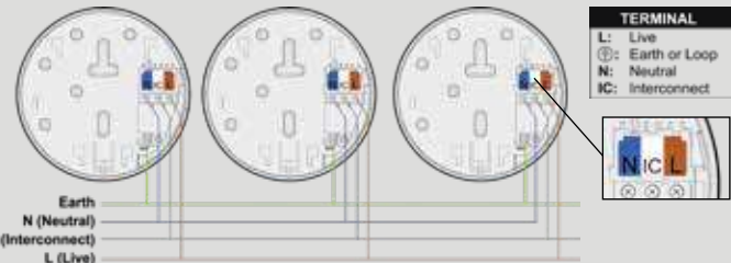
FIG.9 Interconnecting Fire Alarms
