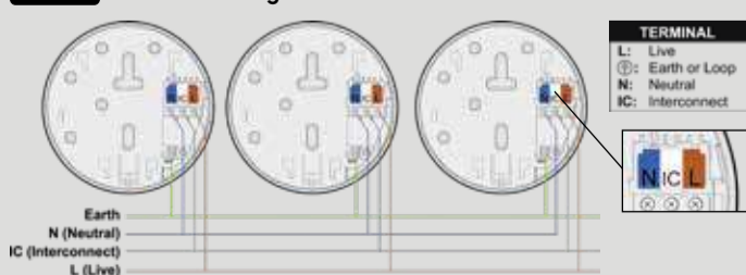
FIG.9 Interconnecting Fire Alarms
