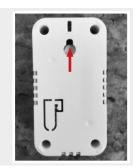
While the red LED is lit on the first alarm, to add other CO alarms to the Home Group, take one from your right and press the TEST/SILENCE button firmly and slowly twice with a pause between taps, so that the red and green LED's flash once with each press. The red LED will then flash 3 times.
