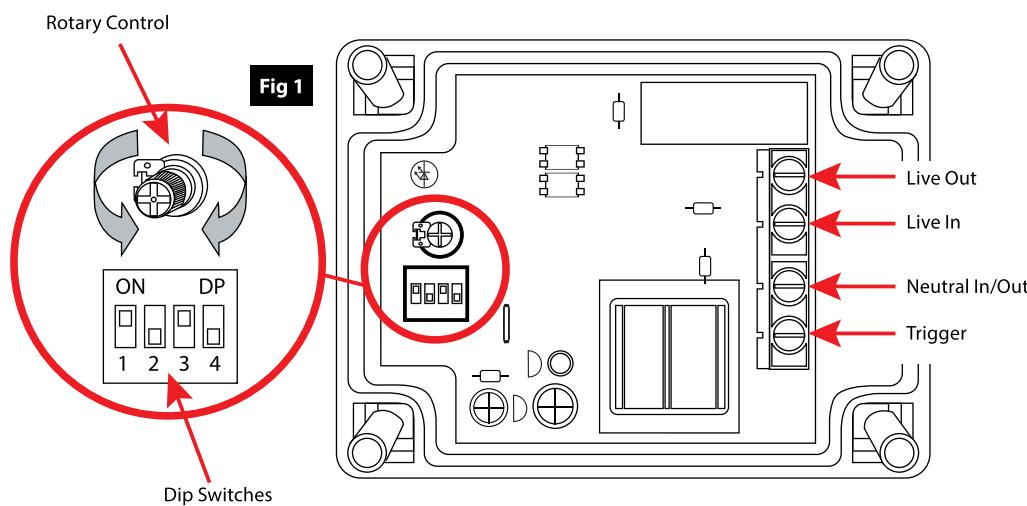
8. Set the desired 'on' time by combination of dip switches and the rotary control, see Fig 1. and table below.
